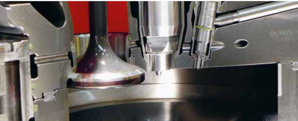
*To ensure that the large engines used in ships and generators meet the strict environmental requirements and emission standards, precise and long-term stable sensors are needed for monitoring and controlling the injection pressure of over 2000 bar.*
