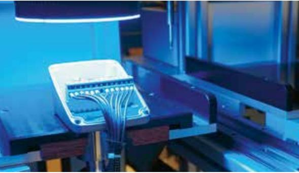
*The SF<sub>6</sub> gas density controllers are set individually and tested for accuracy.*
