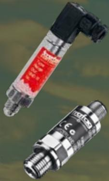
Miniature pressure transmitter: in 1992 Trafag launches the pressure transmitter NA 8891 for industrial applications in the miniature size SW19. The compact size and extremely robust design with fully welded steel housing and thin-film-on-steel sensor will soon become a highly valued solution in mobile hydraulics – from 2012 on meanwhile in its third generation in NAT 8252.
