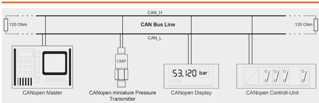
The use of CANopen bus protocol for pressure transmitters allows easier cabling, configuration via bus software, regular condition monitoring of the sensor itself and measurement of pressure and temperature with
