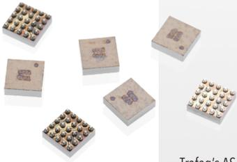
Trafag's ASIC is perfectly tailored to the proprietary sensor elements. The innovative mixed-signal chip with high-performance amplifiers allow best-in-class measuring performance.
