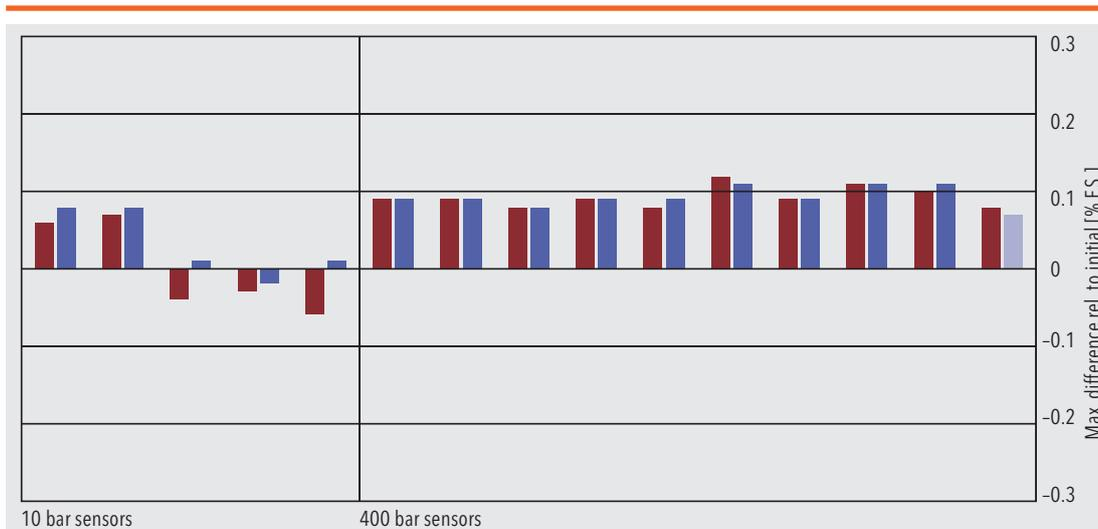
Extreme tests with load changes show that the sensors from Trafag are still stable and usually deviate by less than 0.1 % from the initial value after 10 or 20 million cycles and twice the rated pressure.
