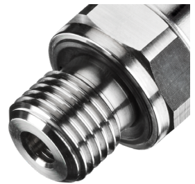
Pressure connection with elastomer seal. The media compatibility as well as the temperature compatibility must be taken into account during selection.
