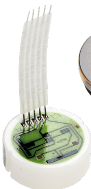
The membrane of the pressure sensor measuring cell is deformed during the pressure measurement. This change leads to a change in the electrical resistance in the resistance elements applied to the membrane. Shown here are the examples of thick-film-on-ceramic (left) and thin-film-on-steel technology (right).
