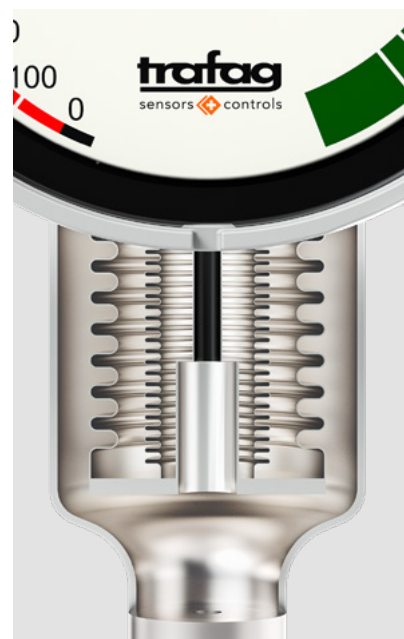
The heart of the 8719 gas density monitor is the advanced reference chamber. It is designed for pressures up to 13 bar.
